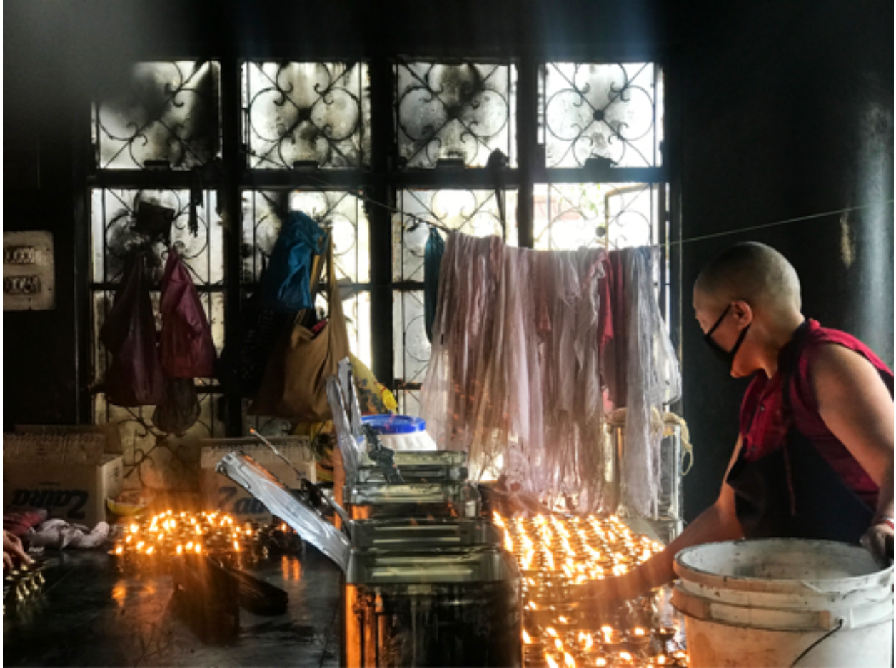
Even inside the butter lamp houses, simple fire safety practices can prevent fires and save lives. Here, the katas are hanging too close to the flames and this is very dangerous.
