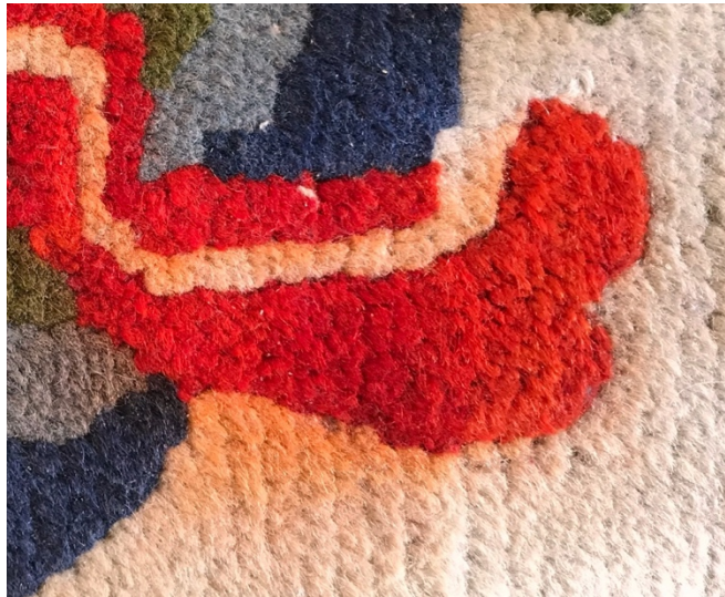
Many paints and dyes are soluble in liquids, sprays, and fumigants. The red color in this carpet was soluble in a water/alcohol solvent cleaning agent.
